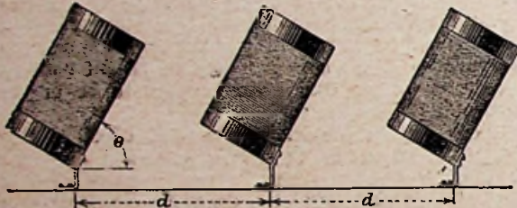
Fig. 1.—To eliminate stray couplings, coils may be supported in this manner.
